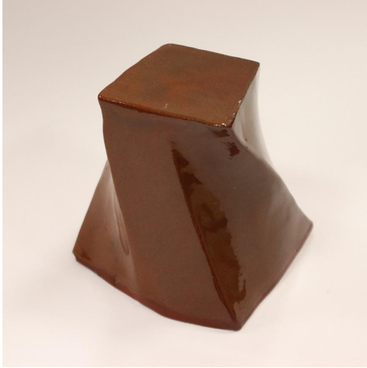
Figure 8. GB5, 8x11x11.5 cm, casting method, red ceramic body, 1100°C (Kum, 2025).
