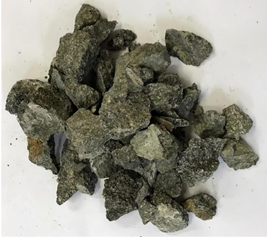
Figure 3. The granite raw material sourced from the Bozüyük District is initially size-reduced (Kum, 2024).
