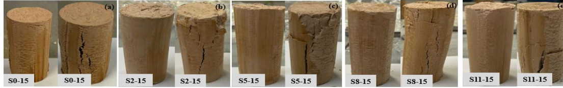
Figure 12. Before and after images of the treated and untreated soils for 15-days curing period (a) without gypsum (S0); (b) S2; (c) S5; (d) S8; (e) S11
