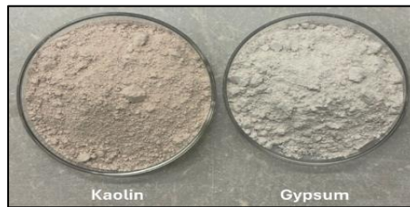
Figure 3. ML type kaolin soil on the left and gypsum on the right
