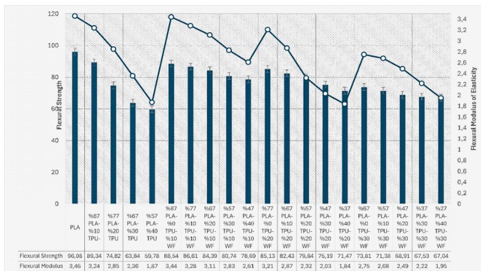
Figure 10. Flexural resistance and elasticity in bending.
