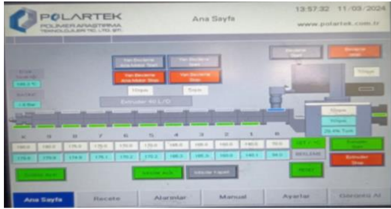
Figure 2. Temperature and feed values applied in the melt mixing process.
