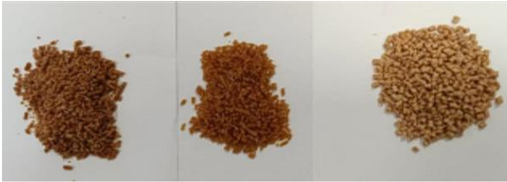
Figure 3. Wood-plastic composites (a) 87-0-10, (b) 77-10-10, (c) 57-30-10.
