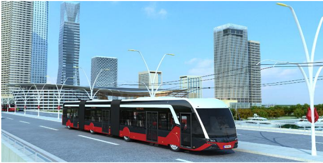
Figure 2. Schematic representation of the dual-mode E-Bus system, capable of operating via overhead catenary infrastructure as well as autonomous battery based propulsion [35].
