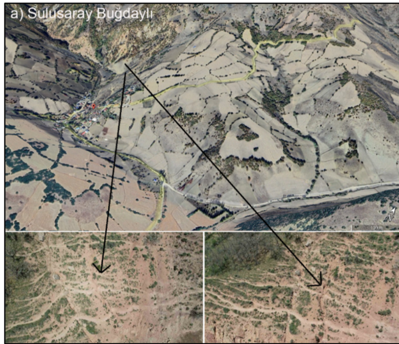
Photo 3. Surface ruptures and ground deformations observed in Tokat province, Sulusaray-Buğdaylı Village.
