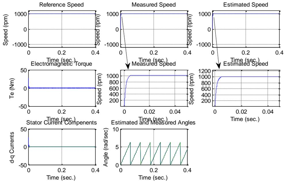
**Figure 14.** Hybrid controller response with step reference signal of PMSM under no load
