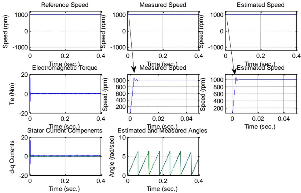
**Figure 11.** Fuzzy logic controller response with step reference signal of PMSM under no load
