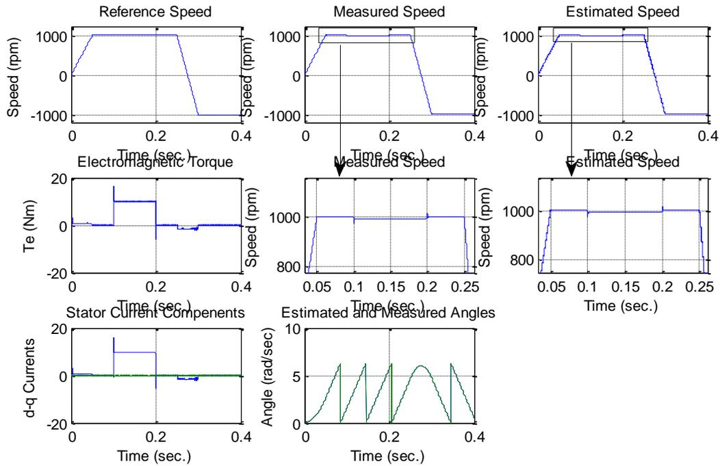
**Figure 16.** Hybrid controller response with variable reference signal of PMSM under load
