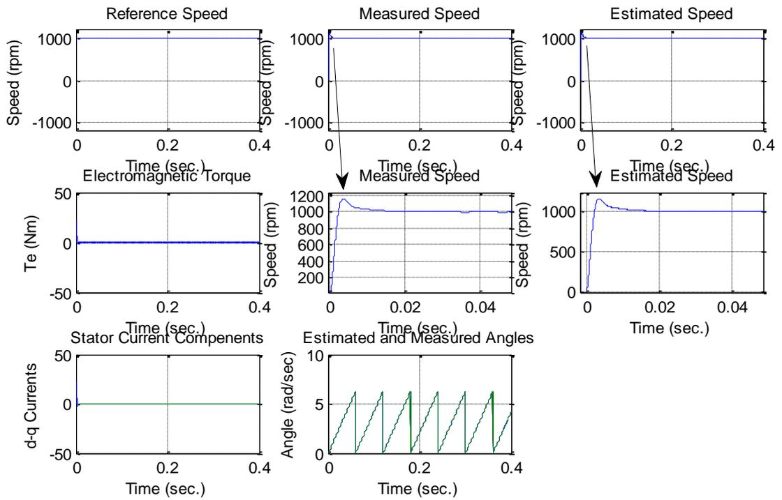
**Figure 8.** PI controller response with step reference signal of PMSM under no load
