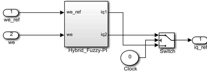
**Figure 2.** Block diagram of the Hybrid speed controller
