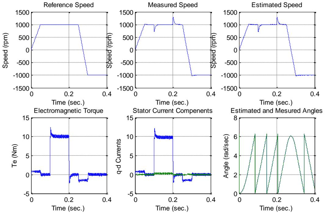
**Figure 10.** PI controller response with given reference signal of PMSM under load
