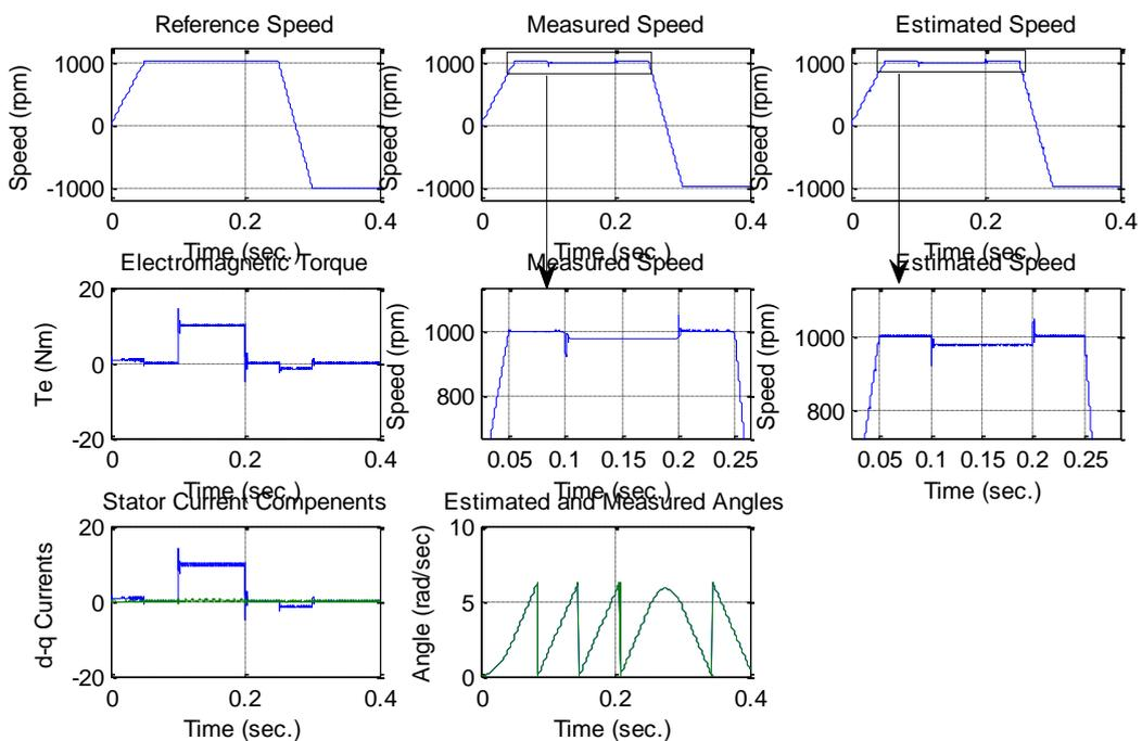
**Figure 13.** Fuzzy logic controller response with given reference signal of PMSM under load
