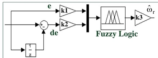
**Figure 3.** Structure of fuzzy logic controller
