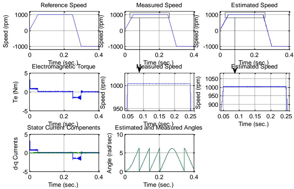
**Figure 15.** Hybrid controller response with variable reference signal of PMSM under no load
