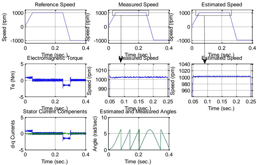
**Figure 12.** Fuzzy logic controller response with given reference signal of PMSM under no load
