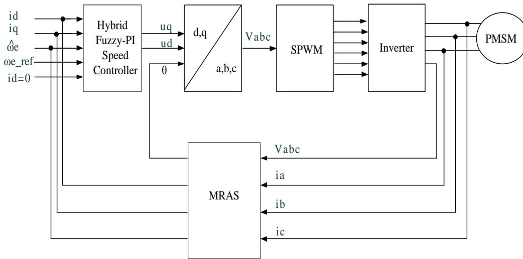
**Figure 1.** Sensorless speed control of PMSM with MRAS
