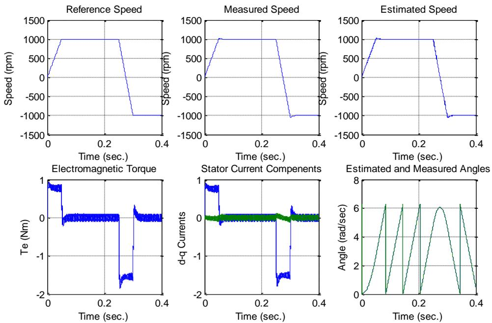
**Figure 9.** PI controller response with given reference signal of PMSM under no load
