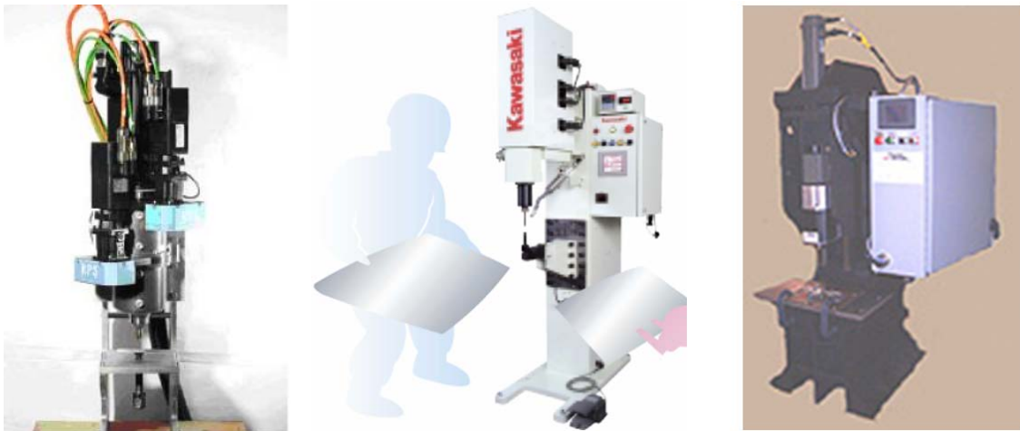
Şekil 4. Solda ve ortada sabit tip, sağda pres tipi SKNK makinası (On the left and in the middle stationary type, on the right press type FSSW machine) [6, 7, 21-23]
