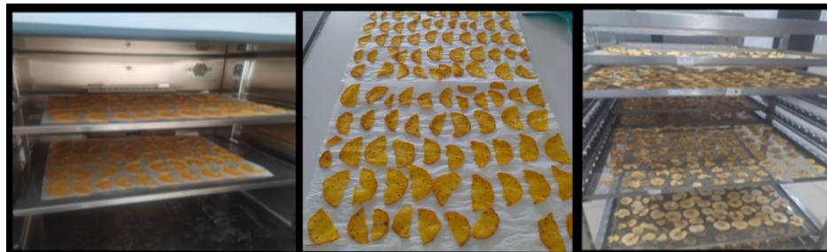
Fig 3. Oven-dried persimmon slices (left), freeze-dried persimmon slices (middle), laser-heated-dried persimmon slices (right)
