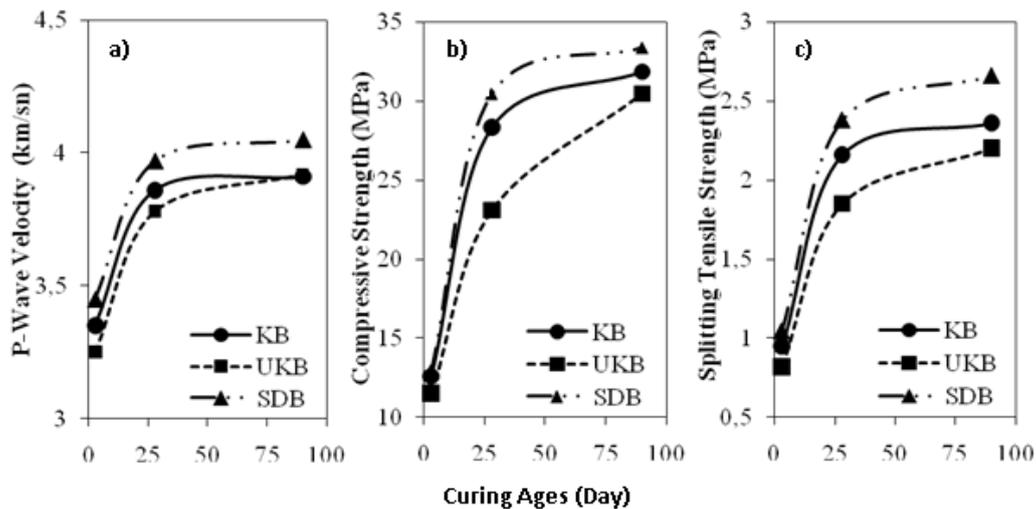
**Figure 1.** Curing Age-P wave velocity, compressive and splitting tensile strength graphs of concrete series
