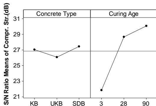
Figure 3. Main effects plot of compressive strength for S/N ratios
