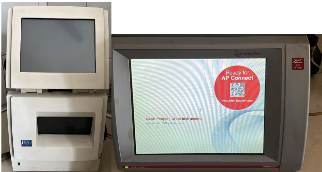
Figure 1. Experimental setup for thermophysical characterization: (a) Rudolph Research Analytical Density Meter for high-precision density readings, and (b) Anton Paar SVM 2001 viscometer used for temperature-dependent dynamic viscosity measurements
