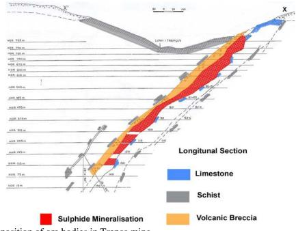
**Figure1**. The position of ore bodies in Trepça mine
