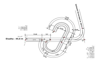
Figure 3.Schematic view of spiral ramp in one level (-45,0m)
