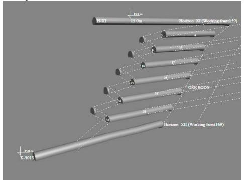
Figure 4. Spiral ramp construction between level XI-XII
