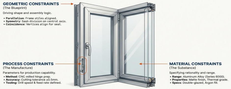
Figure 3 - BIM Hierarchy and Framework for Parameter based selection/decision and model library establishment for the case of a window
