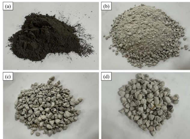
Figure 2. General View of a) Fly Ash; b) 0/4 mm Pumice Aggregate; c) 4/8 mm Pumice Aggregate; d) 8/12 mm Pumice Aggregate
