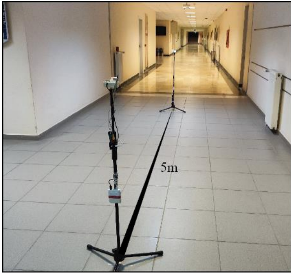
Figure 10. Setup 2: 5m Short-Range Measurement Scenario
