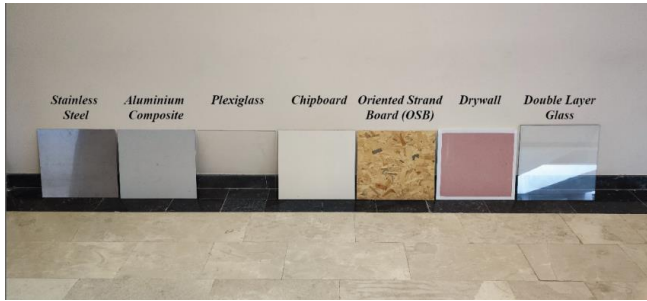
Figure 21. Identification of the Obstacles Used in Experimental Setup 4
