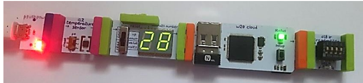
Figure 2. Temperature measurement via Internet
