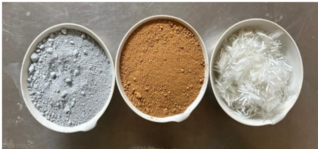
Figure 1. Experimental materials, respectively: Silica fume, Clay, Glass fiber
