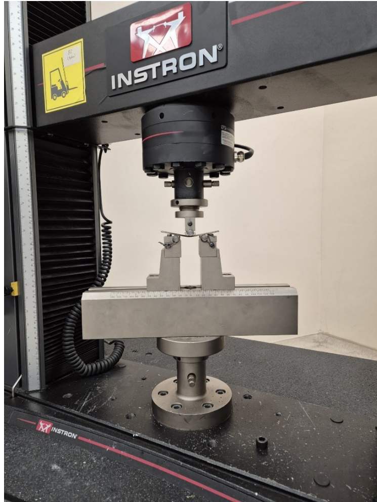
Figure 2. Creep bending test applied to GFRP composites
