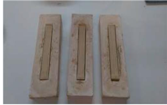
Figure 1. Representative samples formed by the slip casting method.
