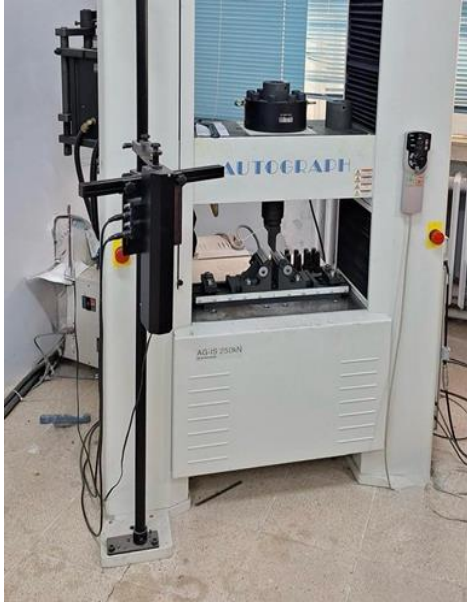
Figure 2. A universal testing machine equipped with a three-point bending fixture.
