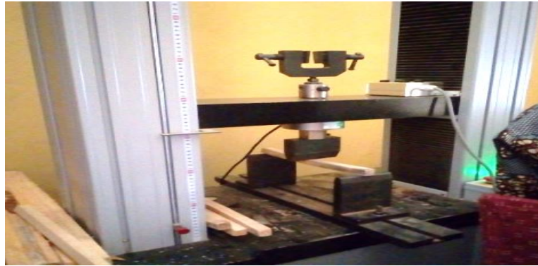
Figure 6. A sample undergoing flexural test in a UTM
