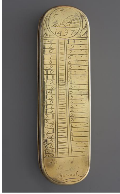
Figure 8: The so-called Holm box shows the perpetual calendar on one side and a table on the other to calculate the speed of the ship 57 .
