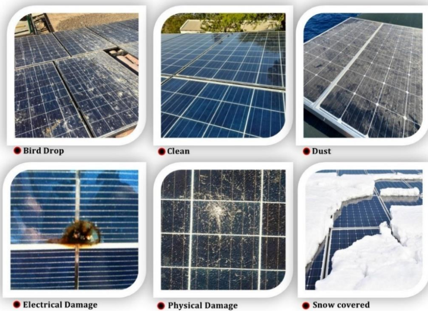
Figure 2. Example images from the PV panel fault detection dataset, showing representative samples for each fault category and the healthy (clean) class
