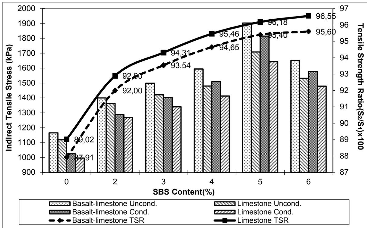
Figure 3. ITS and TSR results for each types aggregates with SBS PMB
