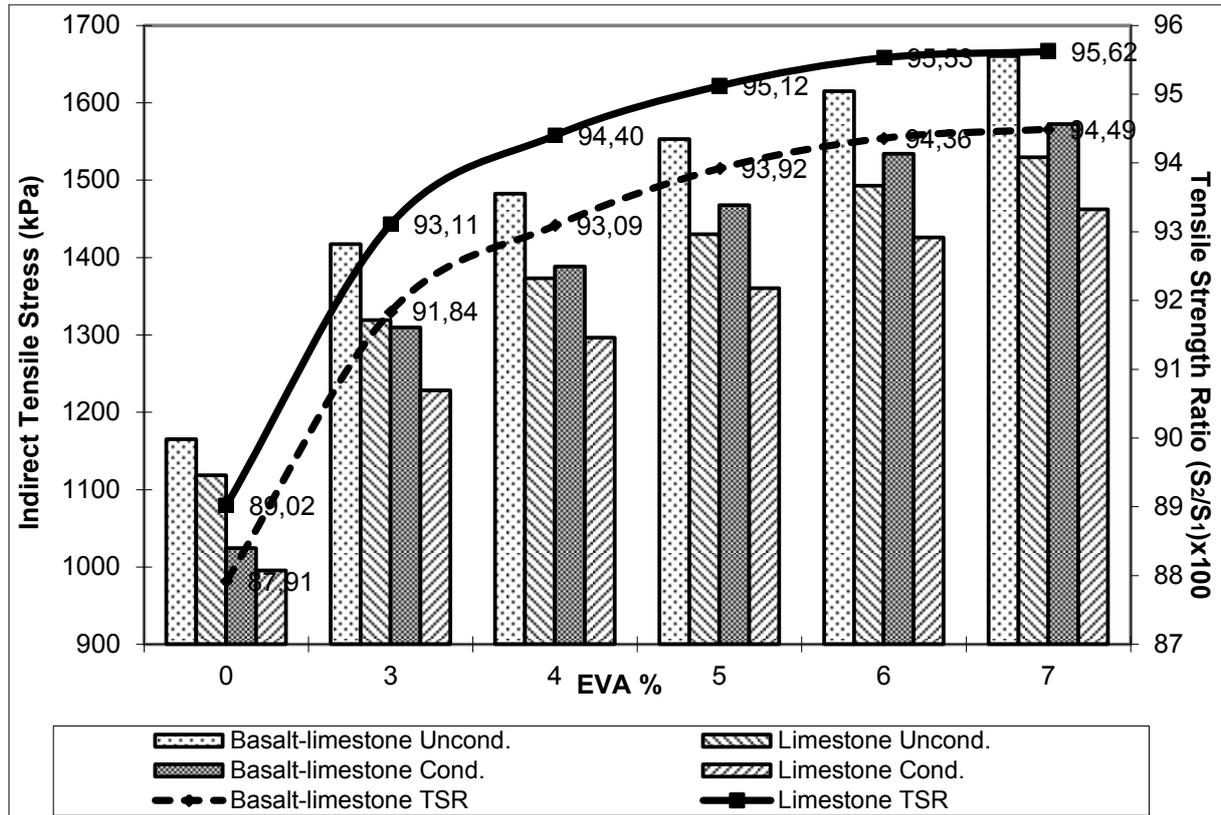
Figure 4. ITS and TSR results for each types aggregates with EVA PMB
