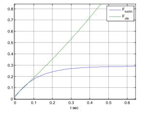
**Figure 5.** Step responses of  $F_{tustin}(z)$  and  $F_{cfe}(z)$  functions
