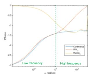
**Figure 2.** Comparison of phase responses of original continuous FOTF, the IIR filter implementation by indirect CFE method (tfcfe<sub>3</sub>) and the IIR filter implementation by direct Tustin recursive method (tftustin<sub>3</sub>).
