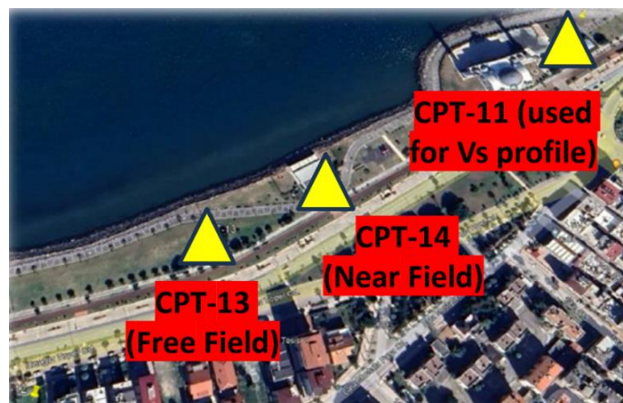
Figure 3. Location of CPT soundings across the study area. CPT-13 (Free Field) and CPT-14 (Near Field) were selected for site response analysis, and CPT-11 was used to derive V_s profiles
