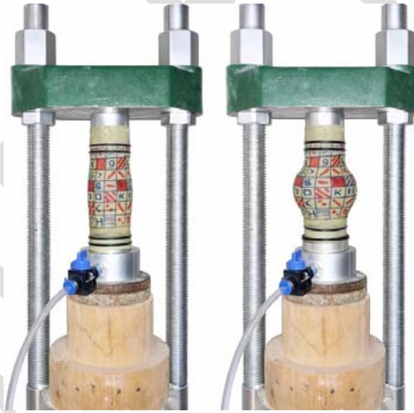
Figure 4 – Soil specimen ready to be loaded axially and subjected to axial strain levels over 40%
