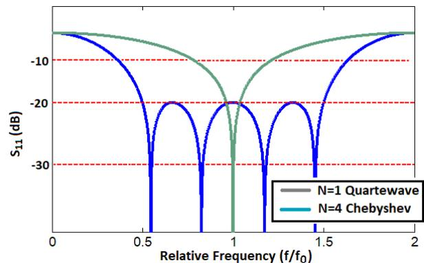
Figure 2. Comparison of reflection graphic between single section (quarter wave) and four-section (N=4) Chebyshev transform
