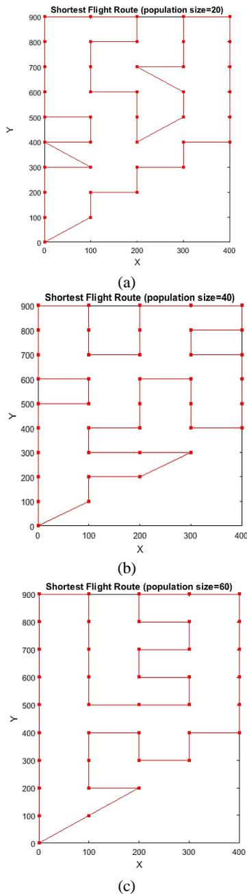
Figure 5. Shortest Flight Routes for Determined Agricultural Land
