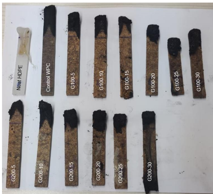
Figure 4. Post-test macrostructural photographs of WPC specimens after the LOI test
