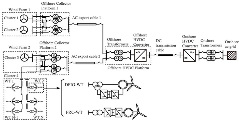
Figure.1. General configuration of an OWPP with two wind farms connected through an HVDC point-to-point link [4]
