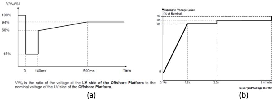
Figure 9. Fault ride through capability required for an (a) offshore wind farm, b) OFTO in the UK [9]
