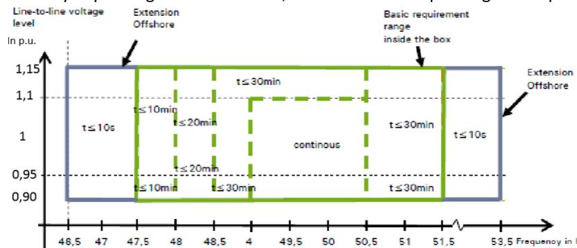
Figure 3. The dimensioning voltages and frequencies in Germany (TenneT) “Offshore”: Duration of operation of a generating unit in dependency of the voltage at the grid connection point and of the nominal frequency [8]
