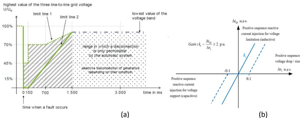
Figure 10 LVRT requirement for (a)the offshore grid connection (b) for the offshore grid connection at the converter level by TenneT [8]
