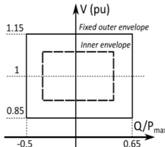
Figure 3 : ENTSOE requirements for voltage at the grid connection point of a dc-connected system [7]
