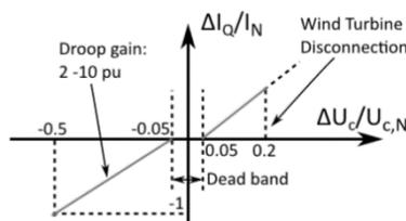
Figure 6: Voltage support during ac fault required by TenneT (Germany) in generating units [8]
