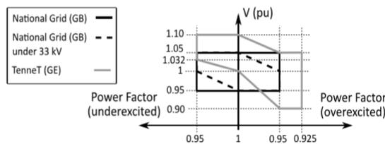
Figure 5: Voltage limits as function of power factor required by National Grid (Great Britain) in WPPs or DC-connected systems and TenneT (Germany) in offshore-connected systems [8,9].
