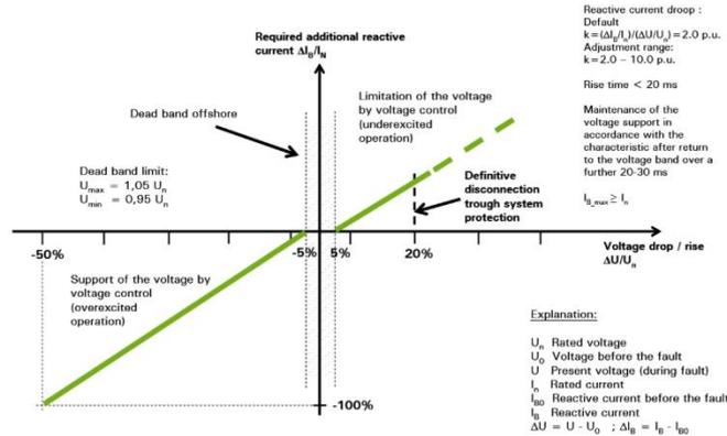
Figure 7 “Offshore”: Principle of the voltage support through each generating unit during grid failures. In individual cases, the gradient of the voltage support can be changed (Reactive current droop with  $k > 2$ ) [8]
