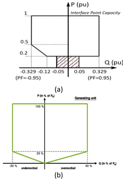
Figure 4 (a) National Grid (Great Britain) requirements for reactive power capacity at the interface connection point of a WPP or a DC-connected system [11], (b) "Offshore": Minimum requirements for the P/Q-operation range of a generation unit within the voltage range of +/- 5% UN (at the generation unit) by TenneT[8,9]
