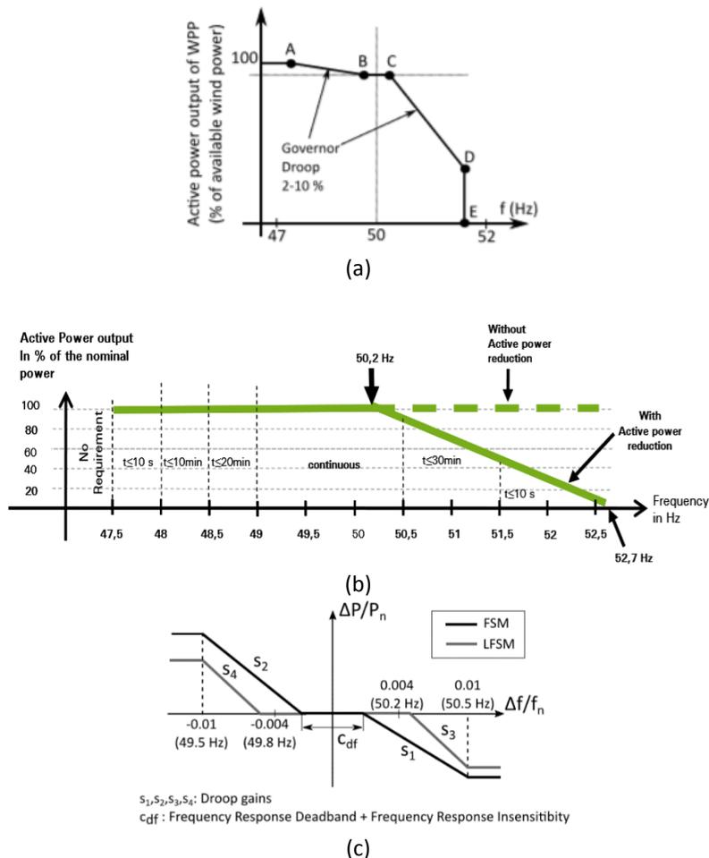
Figure 8. (a) Frequency response characteristic required by EirGrid (Ireland) in WPPs (Points A-E are defined depending on system conditions and location of the OWPP. [4] (b) “Offshore”: Basic Requirement for the active output of a generation unit in dependency to the frequency and to the duration of operation characteristic required by TenneT. [8] (c) ENTSOE requirements for frequency response in DC-connected systems [7]
