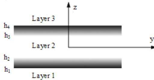
Fig.1. The material variation along the thickness of the FG sandwich plate.
