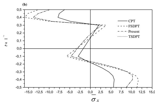
Fig. 3. Comparison of the variation of nondimensional axial stress  $\bar{\sigma}_x$  across the thickness of nonsymmetric FG sandwich plates (2-2-1), ( $k=1.5$ ) by applying different shear deformation theories.
