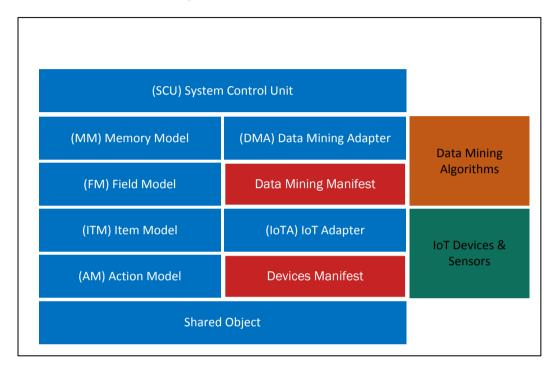
Figure 3. ADLE system architecture
