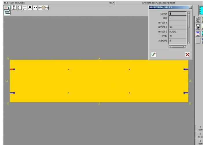
Figure 5. Drilling holes on the lateral constructive parts
