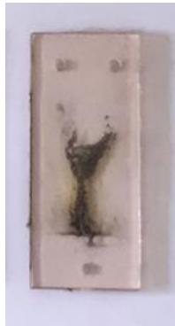
Figure 5. Pure polyester resin sample with carbonized surface tracking.
