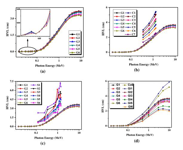
Figure 4. Comparison of half value layers (HVLs) of (a) the studied glass systems with (b) concrete [41] and (c-d) glass samples [39,42].
