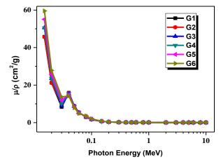
Figure 1. The mass attenuation coefficients  $(cm^2/g)$  of the studied glass systems.
