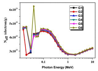
Figure 3. The electron densities  $(N_{eff})$  of the selected glass systems.
