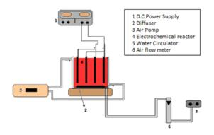
**Figure 2.** Schematic diagram of the electrocoagulation reactor and components.
