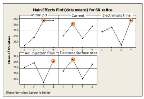
Figure 3. Effects of initial pH, current, electrolysis time, air injection flow and electrode surface area on process performance.
