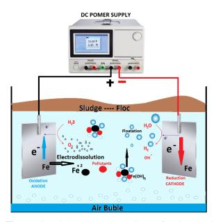
**Figure 1.** Schematic presentation of air-assisted electrocoagulation process.
