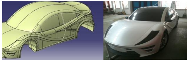
Figure 5. In the Catia package program, the point cloud is created, the surface model is created, and the whole scale of the vehicle, in which a real scale MOCKUP model is produced, is seen.
