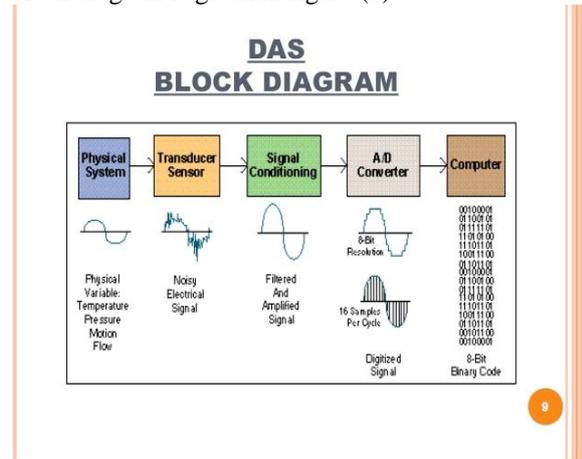
Figure (3)- General Block Diagram of DAQ System
