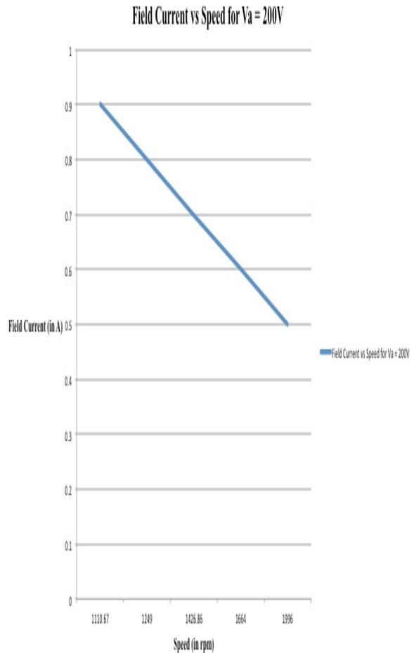
Figure (9) - Field based speed control for  $V_a = 200V$
