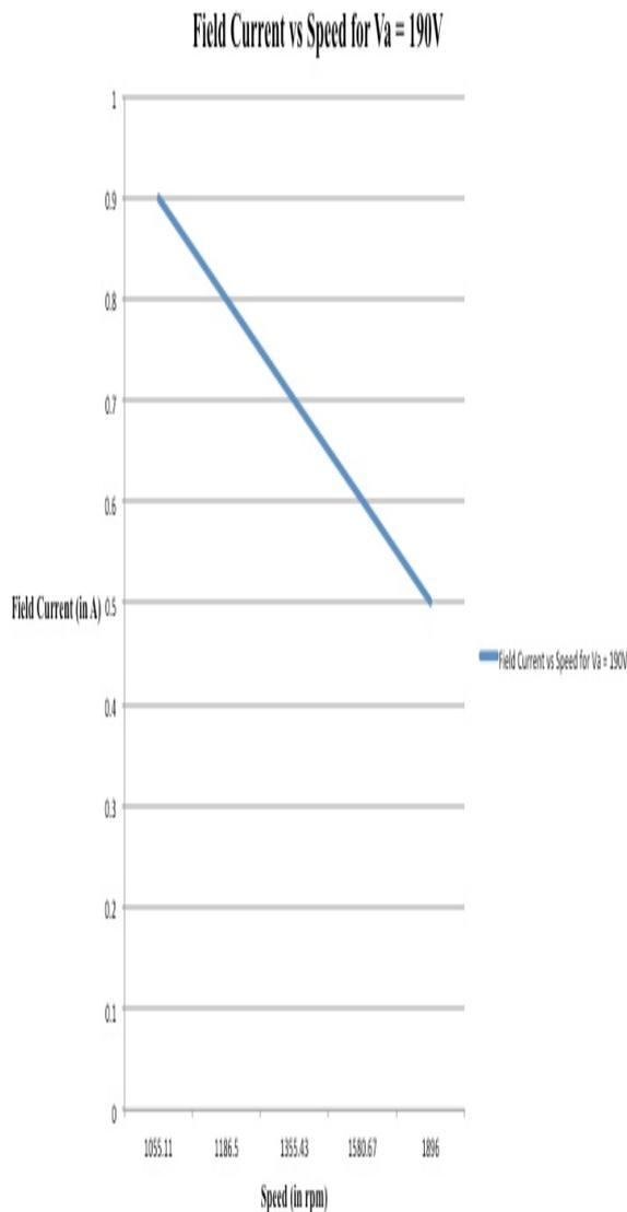
Figure (8) - Field based speed control for  $V_a = 190V$
