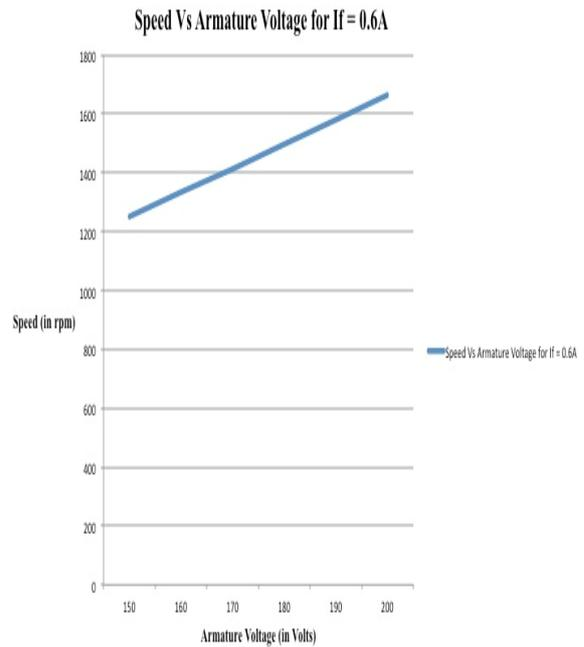
Figure (7) - Armature based speed control for  $I_f = 0.6 A$
