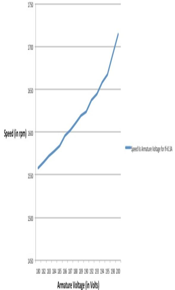
Figure (11) - Armature Control for  $I_f = 0.3A$
