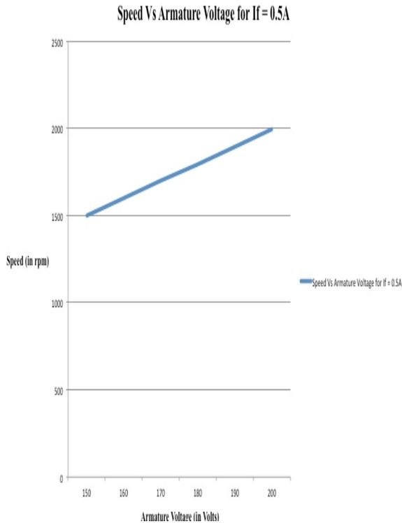
Figure (6)- Armature based speed control for  $I_f = 0.5A$
