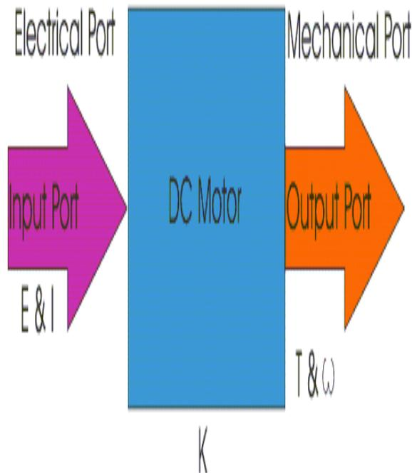
Figure 1. Block Diagram of DC Motor
