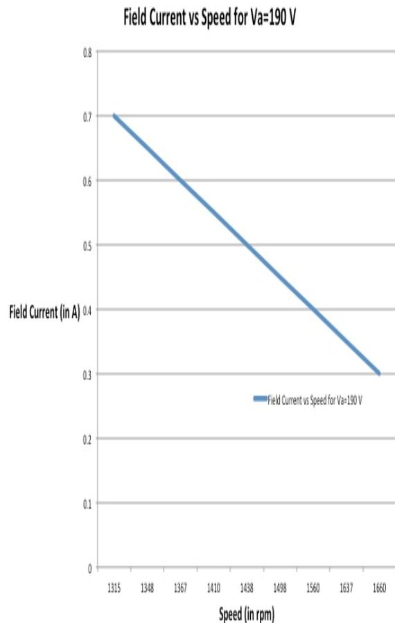
Figure (13) - Field Control for  $V_a = 190V$
