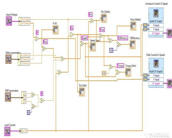
Figure (5) – LabVIEW model for Separately Excited DC Motor.
