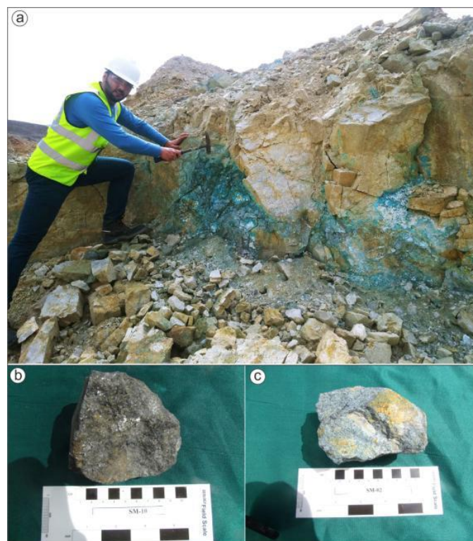
Figure 6. (a) Cu mineralizations (malachite, azurite, covellite etc.) in the quartz porphyry from the Gedabek Au-Cu deposit, (b) chalcopyrite and sphalerite (c) malachite and covellite in hand samples.
