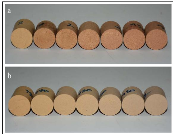
Figure 4- a\*) SFA-containing brick samples sintered at 950°C
