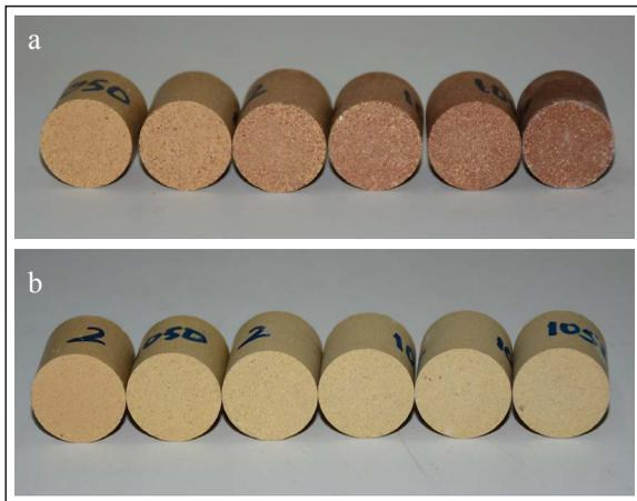
Figure 3- a\*) SFA-containing brick samples sintered at 1050°C
