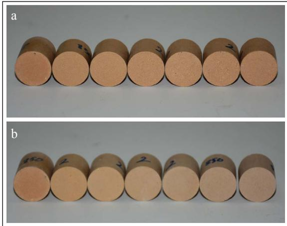
Figure 5- a\*) SFA-containing brick samples sintered at 850°C\*The figure shows the brick samples containing 0% fly ash on the left hand and 60% fly ash on the right hand, so the fly ash content increases from left to the right. b\*) SFA-containing brick samples sintered at 850°C\*The figure shows the brick samples containing 0% fly ash on the left hand and 60% fly ash on the right hand, so the fly ash content increases from left to the right.
