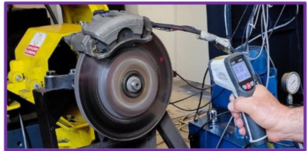
Figure 7. Verification of disk temperature measurement.
