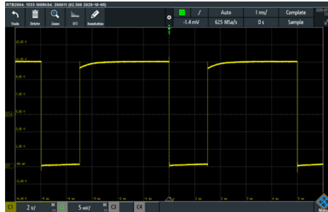
Figure 8. Motor End PWM Signal-Reverse Direction
