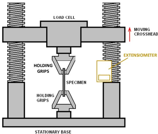
Figure 2. Tension test procedure
