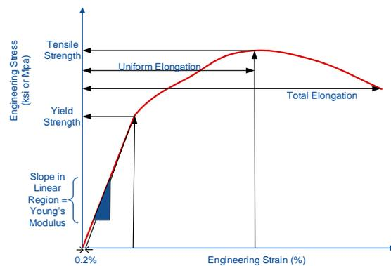
Figure 3. Stress-strain graph
