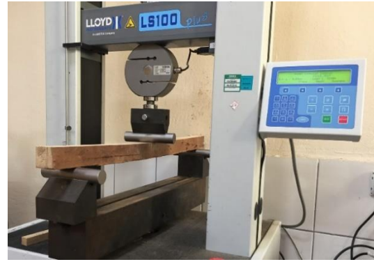
Fig. 5. Bending test set-up
