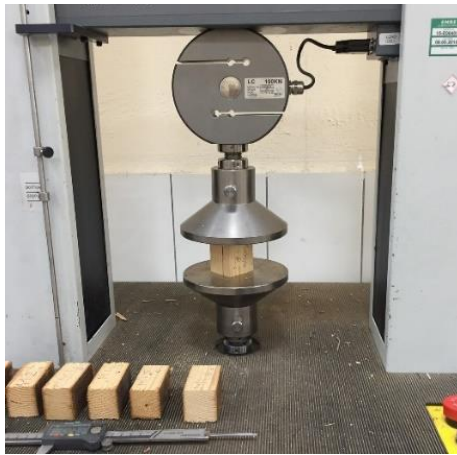
Fig. 6. Compression test parallel to the grain
