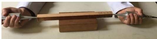
Fig. 4. Ultrasound measurement on a small specimen
