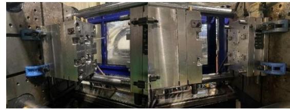
Figure 3. Plastic injection mold female and male plates.
