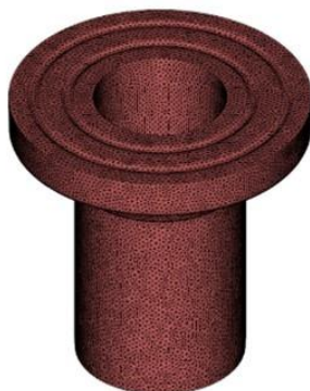
Figure 4. Mesh structure used in MoldFlow analysis.
