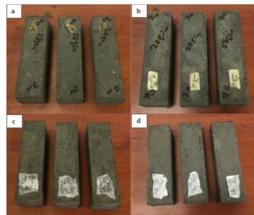
Figure 2. Appearance of the geopolymer samples after 48 hours of curing a)W1-S, b)W2-S, c)W1-EP, d)W2-EP
