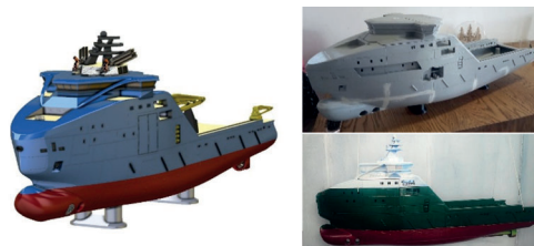
Figure 3: Arctic class ocean-going tug 3D model with complex hull lines, fine details, and printed project (Author's work).
