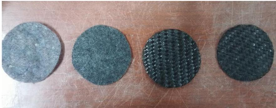
**Figure 1.** Different types of geotextiles used in the experiments (from left to right: the non-woven geotextiles G1, G2; the woven geotextiles, G3 and G4)
