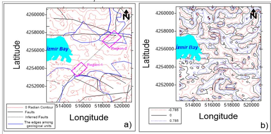
**Figure 7.** a) Comparison of TAHG results with the edges b) TAHG results dashed lines show the 0-radian contour of the tilt angle. blue lines are contours of the tilt angle for  $-\pi/4$  radian and red lines are contours of the tilt angle for  $+\pi/4$  radian.
