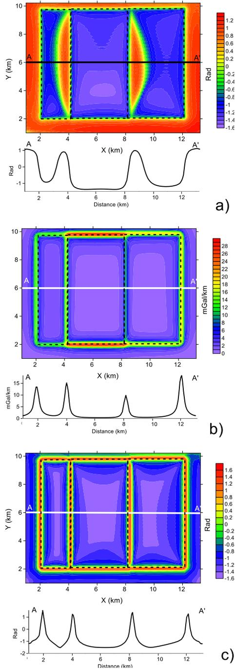
**Figure 2.** The gravity anomaly map and edge detection results a) TA-Tilt angle b) the THDR-the total horizontal derivative, c) TAHG-tilt angle of the total horizontal gradient.
