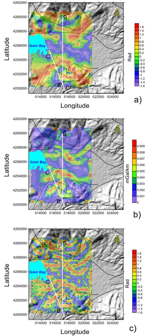
**Figure 5.** The gravity anomaly map and edge detection results a) TA (Dashed lines indicate the 0-radian contour) b) the THDR c) TAHD (Dashed lines indicate the 0-radian contour)
