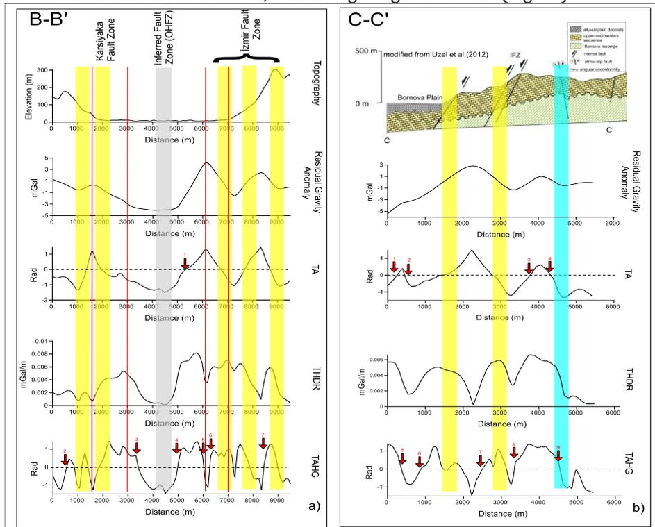
**Figure 6.** The Cross sections on topography map, the residual gravity anomaly map and edge TA, THDR, TAHG (Red lines indicate the edge of geological units; Yellow lines indicate the known fault zones; Blue lines indicate the strike-slip fault zone; Gray lines indicate the Inferred fault zone (OHFZ) Red arrow lines indicate the possible edges) a) B-B' cross section b) C-C' cross section
