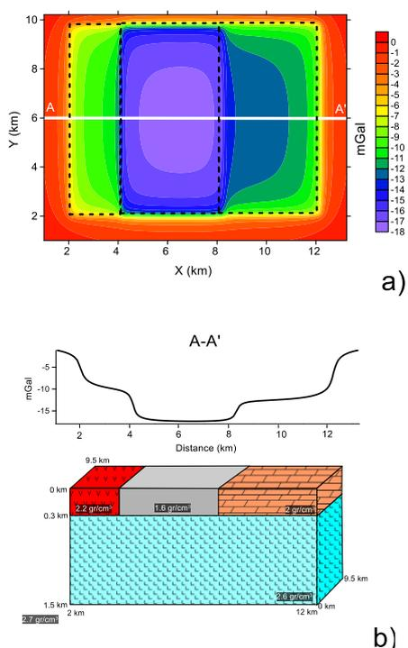
**Figure 1.** Representation of a) theoretical gravity anomaly maps (dashed line shows edge of prisms) b) the plan of the vertical prism models and A-A' cross section in theoretical gravity anomaly maps.
