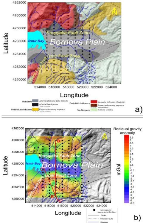
**Figure 4.** a) Geology map of the study area (modified from Uzel et al., 2012) b) Residual gravity anomaly map obtained by using 2nd degree trend analysis which subtracted from Bouguer gravity anomaly map of the study area.
