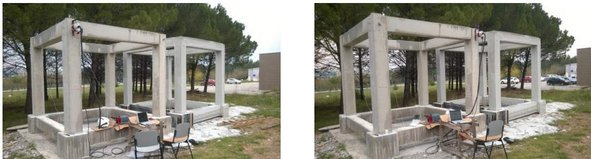
Figure 7. Two positions in one direction of the electrodynamic shaker on NF.
