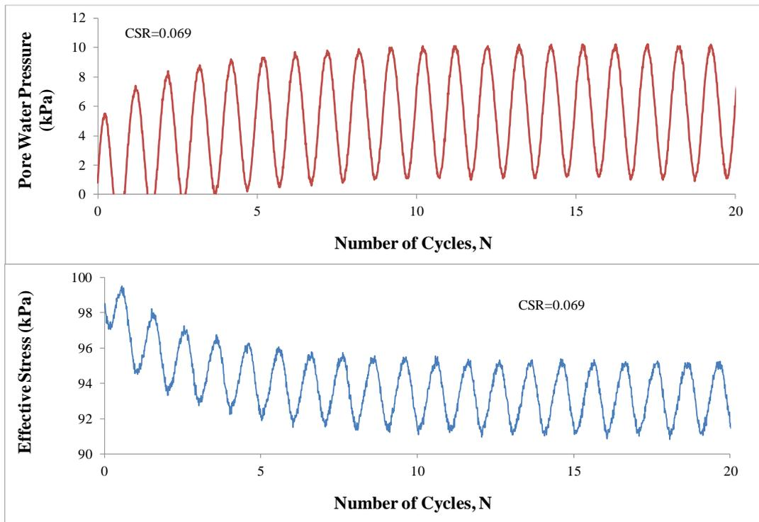
Figure 4. The change of pore water pressure and effective stress for  $D_r=80\%$  and  $CSR=0.069$  with number of cycles.
