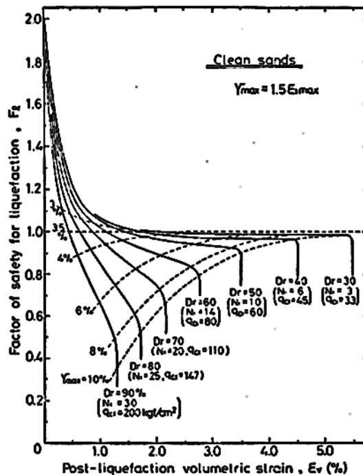
Figure 2. The relationship between post liquefaction volumetric strain and factor of safety (Ishihara and Yoshimine, 1992).
