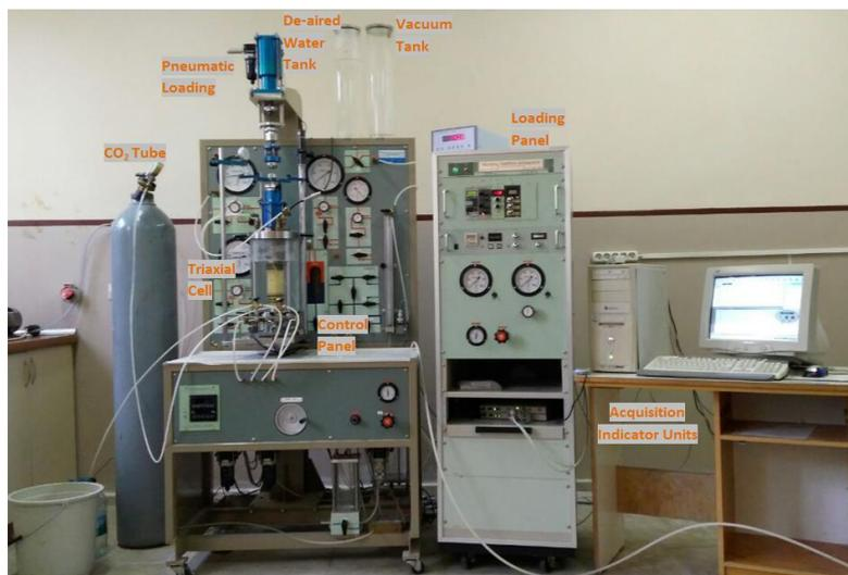
Figure 3. Dynamic Triaxial Test System
