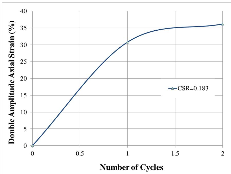
Figure 9. The change of double amplitude of axial strain with number of cycles for  $D_r=80\%$  and  $CSR=0.183$ .
