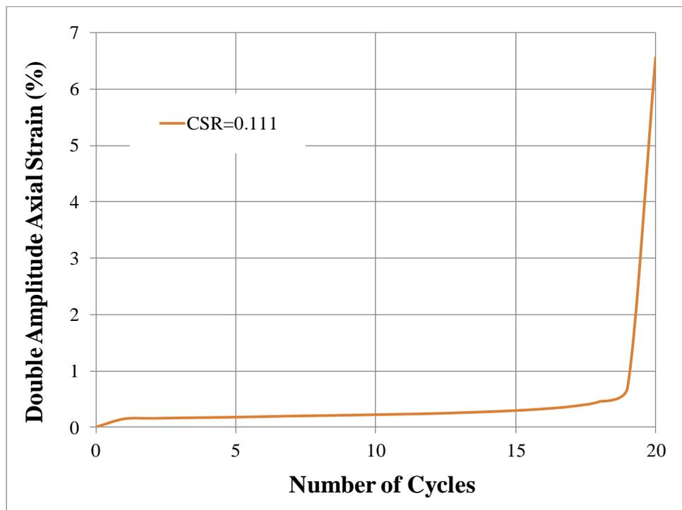
Figure 7. The change of double amplitude axial strain with number of cycles for  $D_r=80\%$  and  $CSR=0.111$ .
