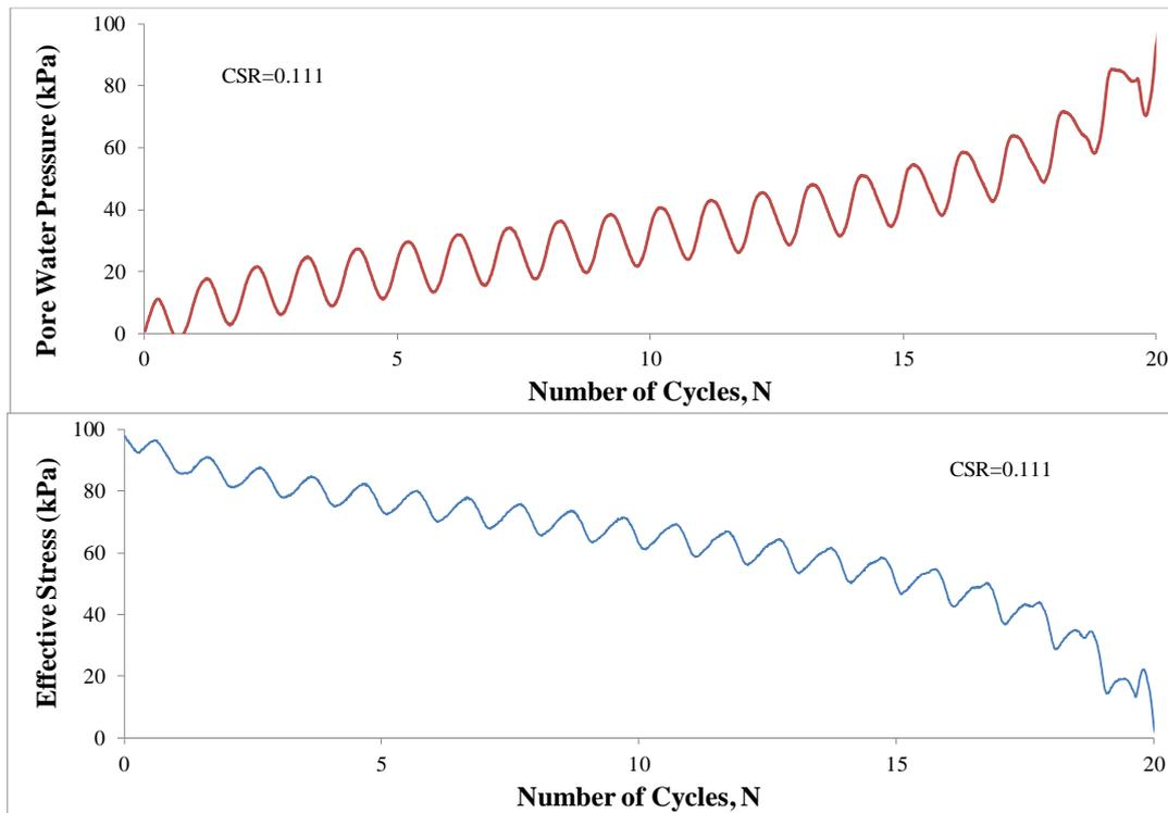
Figure 6. The change of pore water pressure and effective stress for  $D_r=80\%$  and  $CSR=0.111$  with increasing number of cycles.
