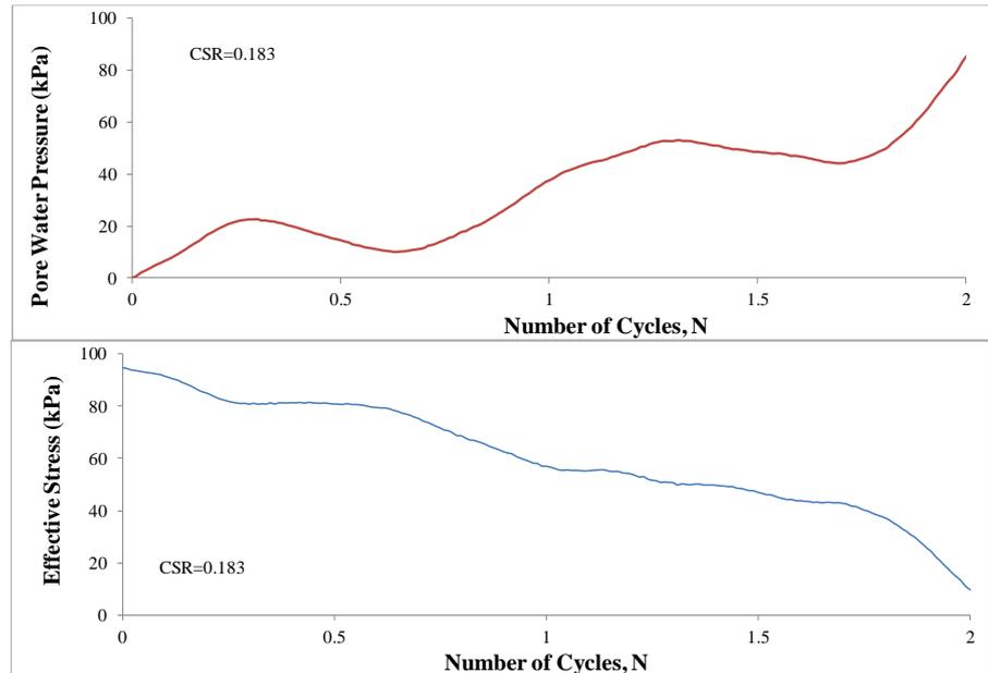
Figure 8. The change of pore water pressure and effective stress for  $D_r=80\%$  and  $CSR=0.183$  with number of cycles.
