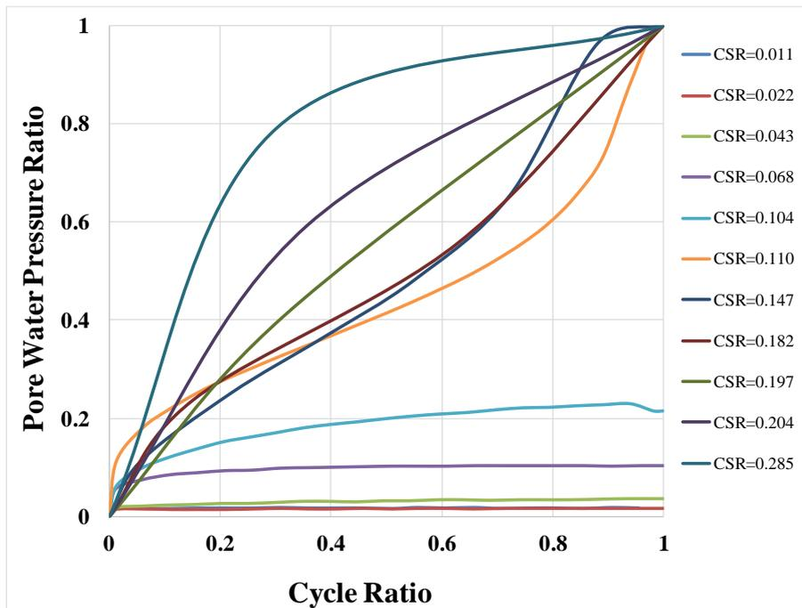
Figure 12. Rate of pore water pressure ratio build up with cycle ratio
