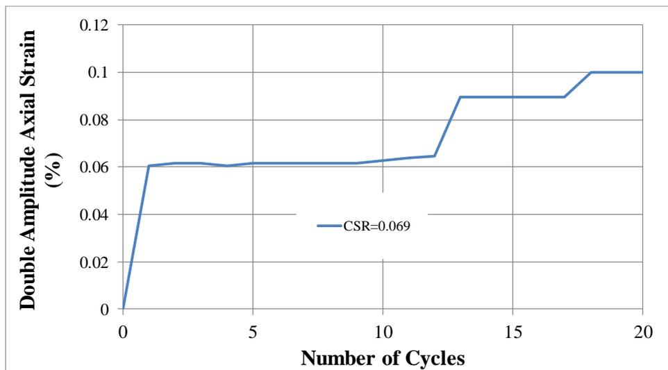
Figure 5. The change of DA with number of cycles for  $D_r=80\%$  and  $CSR=0.069$ .
