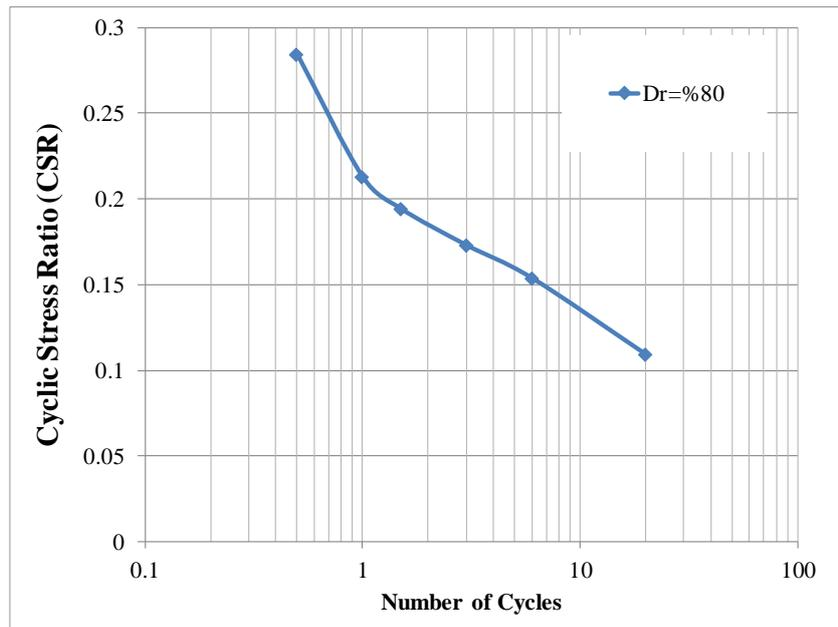
**Figure 10.** Plot of CSR with number of cycles to liquefaction for  $D_r=80\%$
