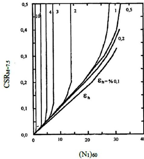
Figure 1. Volumetric strain values by using cyclic stress ratio and SPT on saturated sands (Tokimatsu and Seed, 1987)
